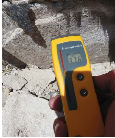
Figure 1. Though it looked sound from the outside, the manufactured-stone veneer on this nine-month-old house was absorbing water and soaking the mortar base coat (left) and the sheathing and framing underneath. The only way to fix the problem was to pull off the stone (right) and install a proper substrate.
